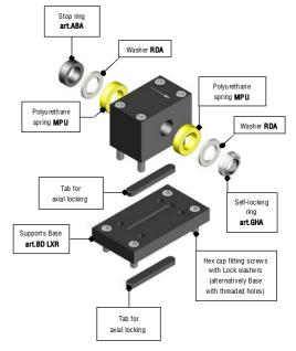
Fitting on machine with Supports Base above
