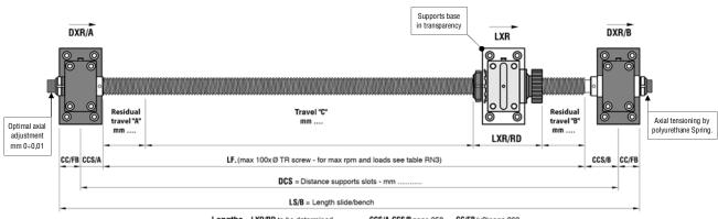
• TRAPEZOIDAL SCREW DESIGN made from our IF threaded bar and predisposed for Rotary Nut supports.
