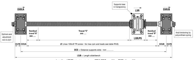
Lengths = LXR/PS to be determined .......CCS/A-CCS/B page 258 CC/FB (x2)page 262 (the length LXR/PS has to be determined for every individual project and normally is substituted with the length of the entire carriage)
